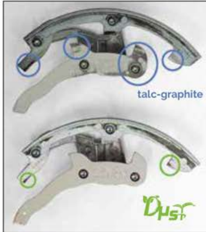
Figure 12. Wear differences on seed singulator of the CNH seed meter when using talc-graphite and DUST™.
